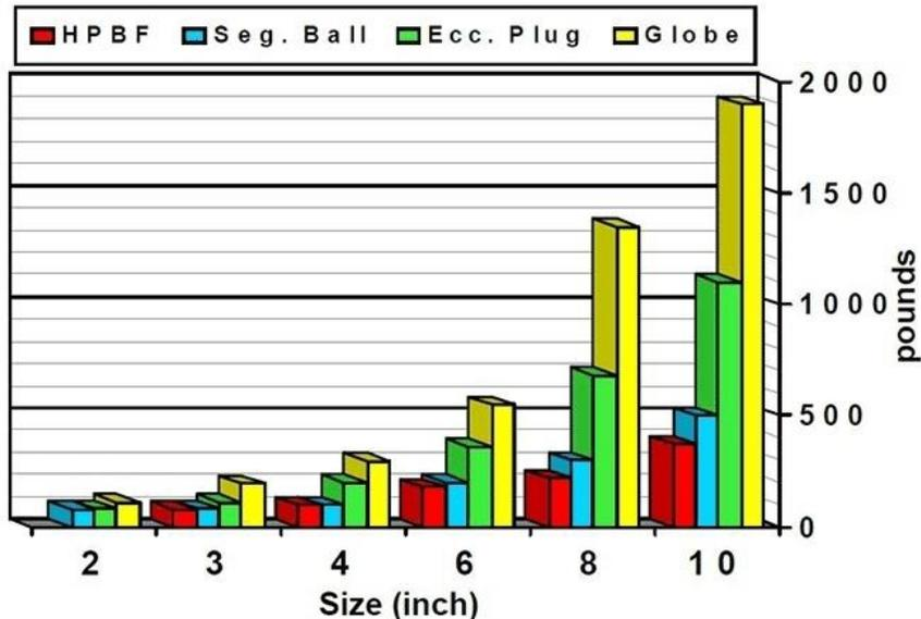
**Figure 2: Control valve weight comparison**
