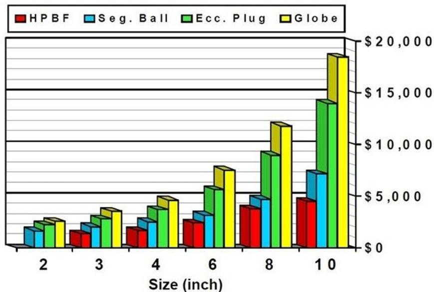
**Figure 1: Control valve cost comparison**
