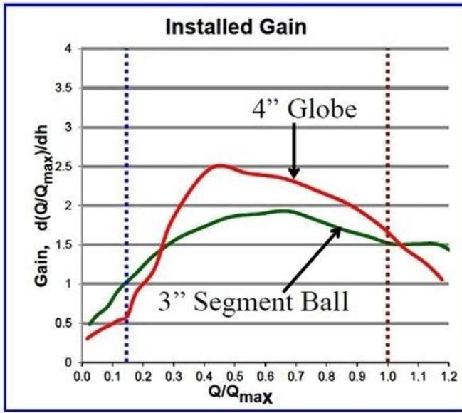
**Figure 7: Comparison of the installed gain of two different valves in the same system.**
