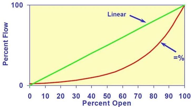
**Figure 5. Ideal inherent flow characteristics**
