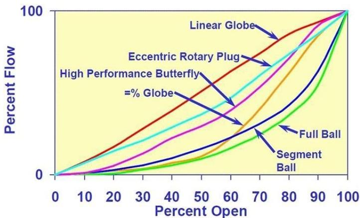
**Figure 6. Typical inherent flow characteristics**
