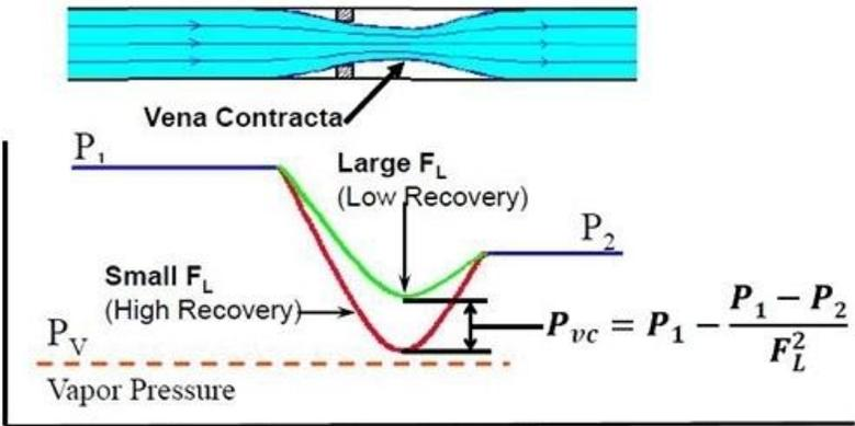
**Figure 3: Behavior of liquid pressure inside a control valve**
