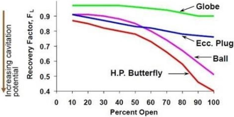
**Figure 4: Liquid pressure recovery factor**
